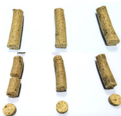
Fig. 2. Examples of broken pellet samples: top– in the first day; bottom – when they broke during the monitoring period
